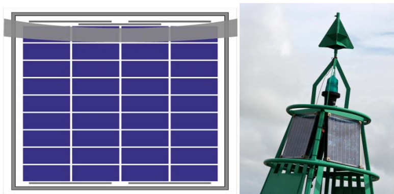
Figure 4 Power reduction approximately 90% due to shadow
